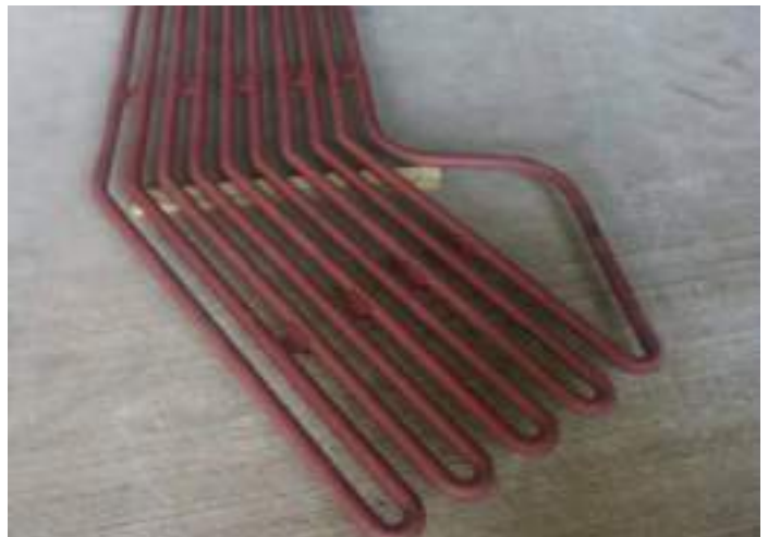
Super Heater Coils | SA 213, Gr T11, Alloy Steel
